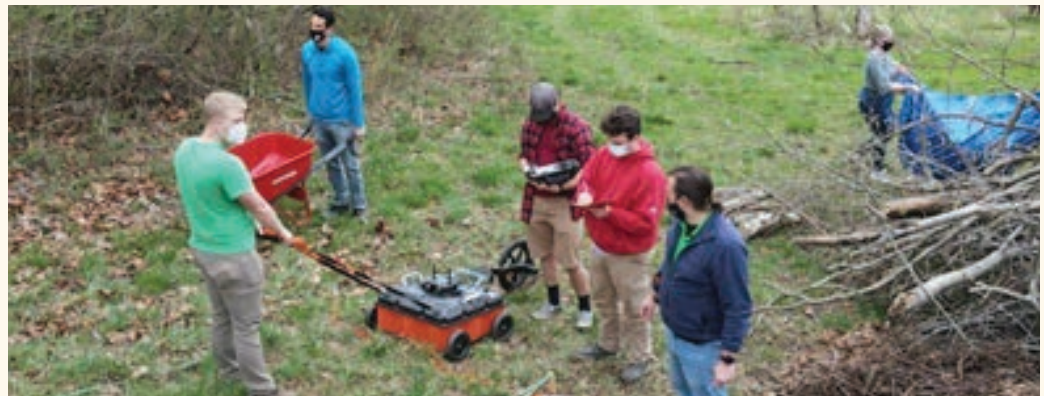
Figure 3 – Marshall University Civil Engineering Students Using GPR to Map Graves
