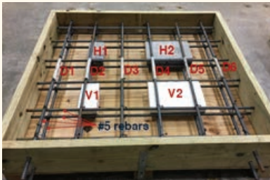
Reinforced concrete slab with artificial voids, debonding and honeycomb.
