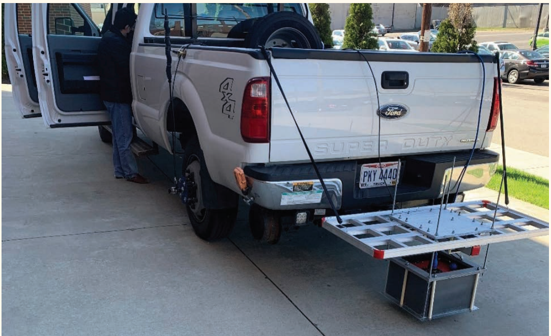
MU Hi-rail currently being equipped with GPR instrumentation for testing on the rail lines.
