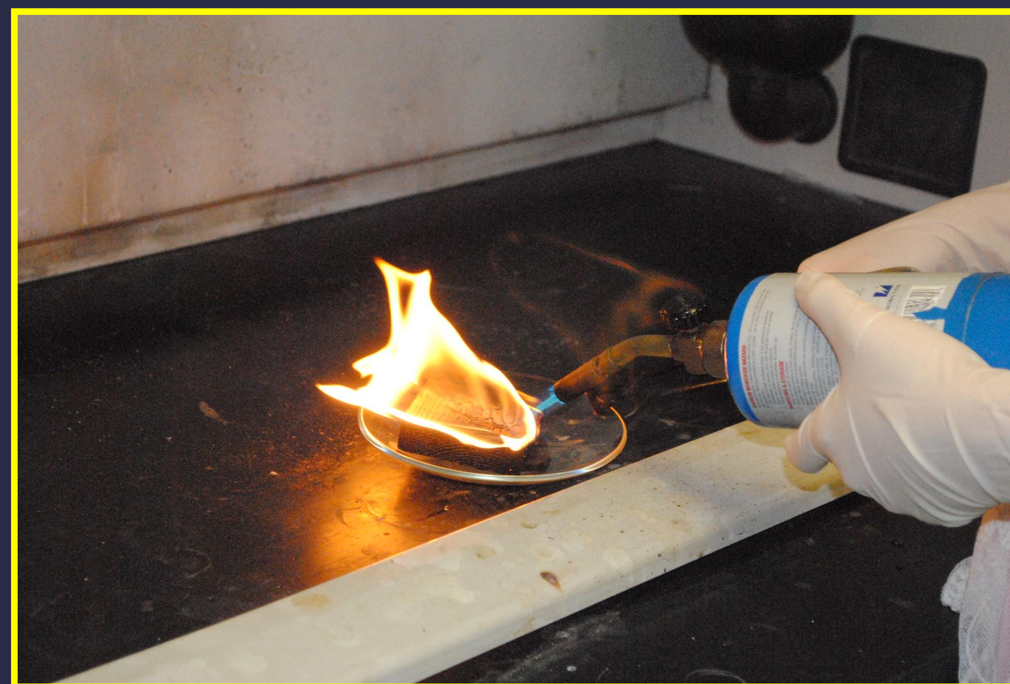
Figure 1. Charring process for wood samples.
