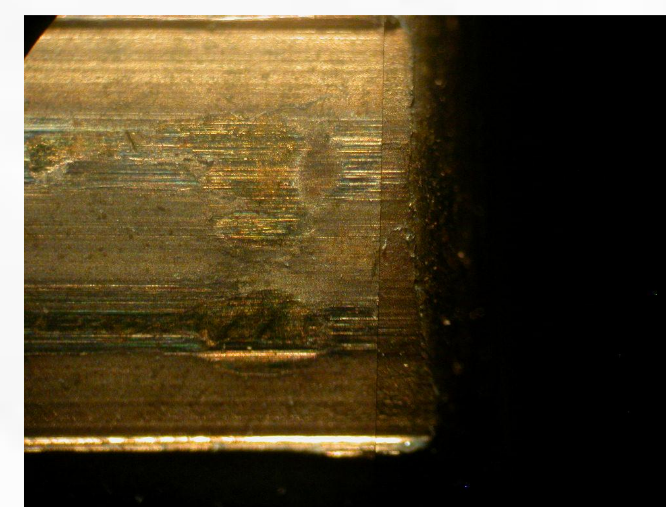
Before (left) and after (right) 1000 bronze brush cycles (S&W)
