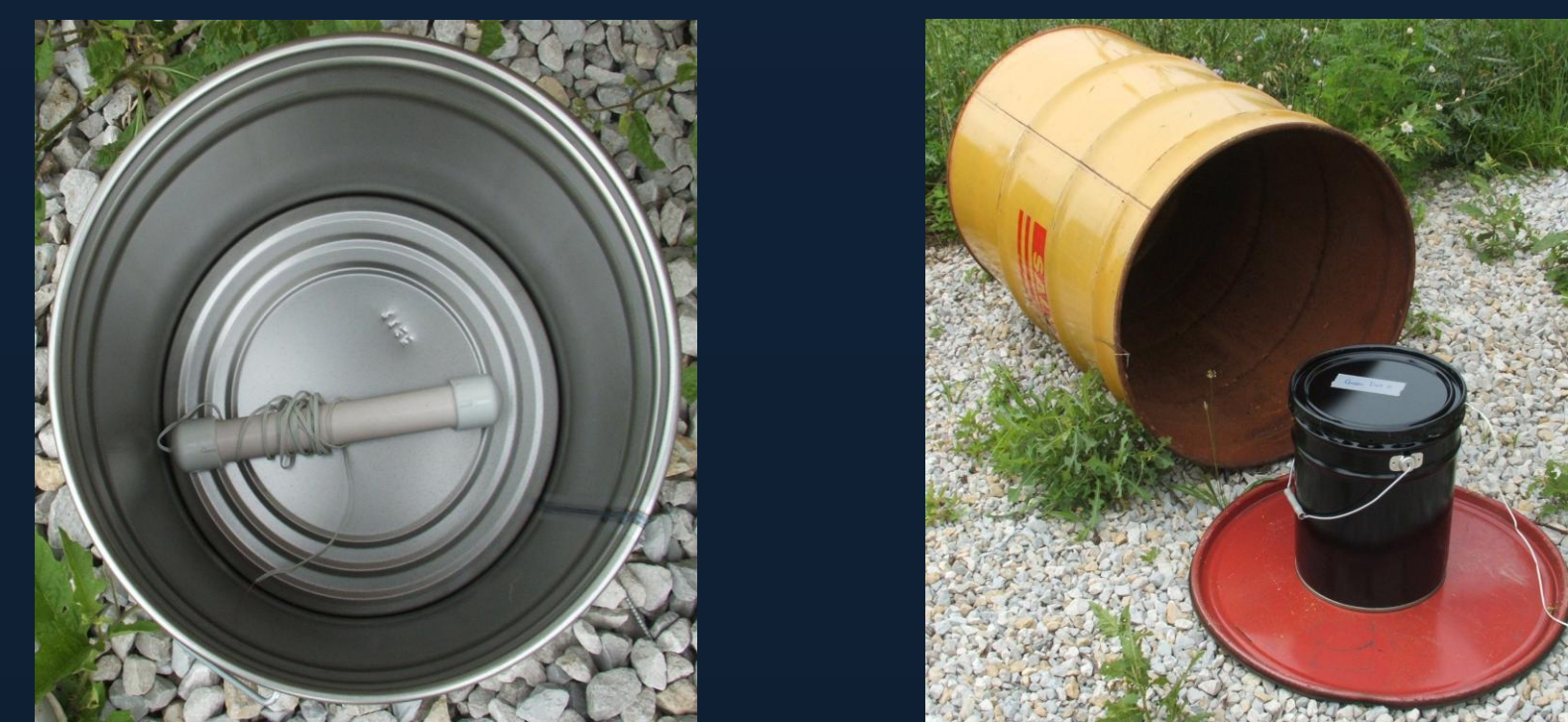
Figure 1: A unexploded pipe bomb with an electric match in a 5 gallon bucket (left), and a 55 gallon barrel used to contain the explosion in a safe environment (right).
