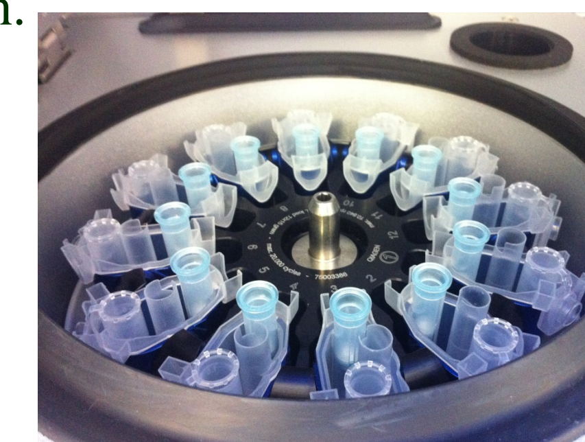
Figure 5 The Qiagen® QIAcube®: centrifuge holding samples (6)
