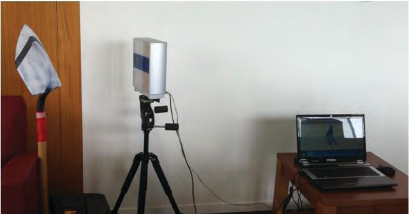
Figure 3: The NextEngine 3D Laser Scanner was set up on a tripod and attached to a laptop computer featuring the software ScanStudio HD. The shovel was held up and positioned 30cm in front of the scanner.
