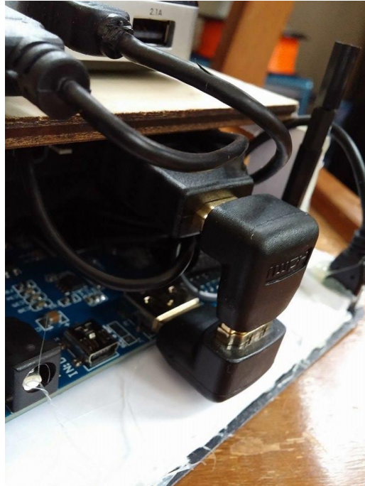
Figure 7. The above figure demonstrates the HDMI adapters used for the screen and Raspberry Pi connection.
