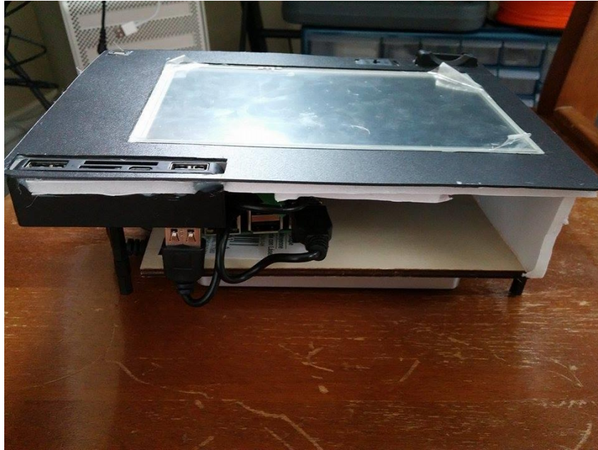
Figure 11. The outside ports were glued into the plastic desk pad as shown above.
