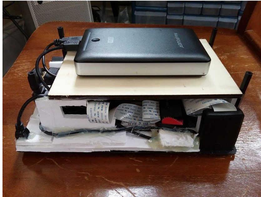
Figure 9. The battery was glued to the board as shown above.
