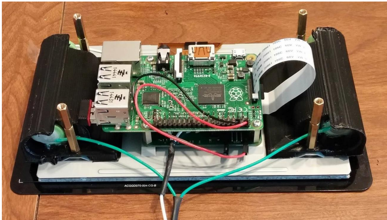
Figure 19. The Raspberry Pi 2 and batteries were attached to the screen using standoffs as shown above.
