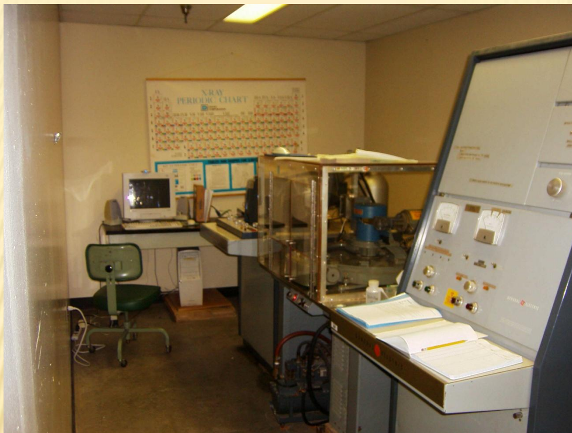
General Electric X-ray diffractometer (XRD-9000 Z-80/ XRD-6VS) & XRF Spectrometer (1960's model upgraded in 1986).
