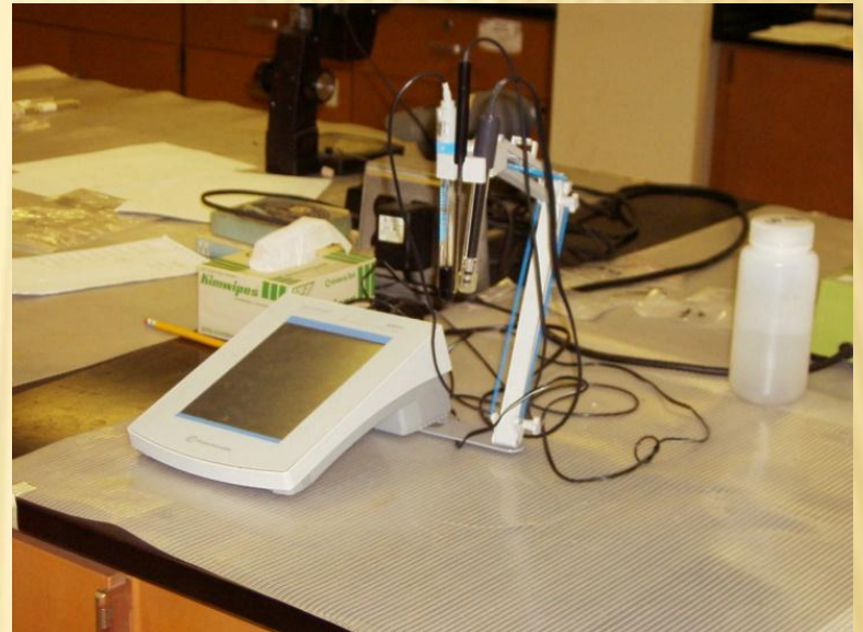
Acumet AR-50 pH and conductivity meter
