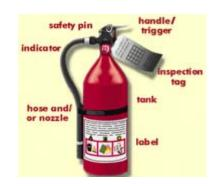
The pressure should be within the recommended level on extinguishers equipped with a gauge. The needle should be in the green zone. If the needle is not in green zone, the extinguisher requires professional maintenance; report this information to the Department of Safety & Health (696-2993).
