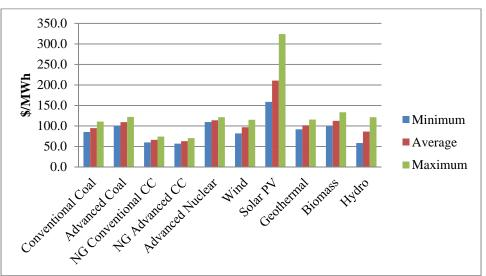
Figure 9: Estimated Levelized Cost of New Generation Power Plants<sup>136</sup>
