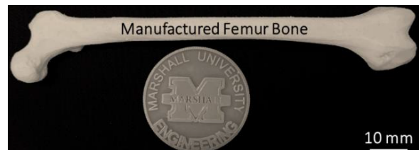
Figure 1: An X-ray \mu -CT-based, biocompatible femur bone model fabricated at Marshall University.
