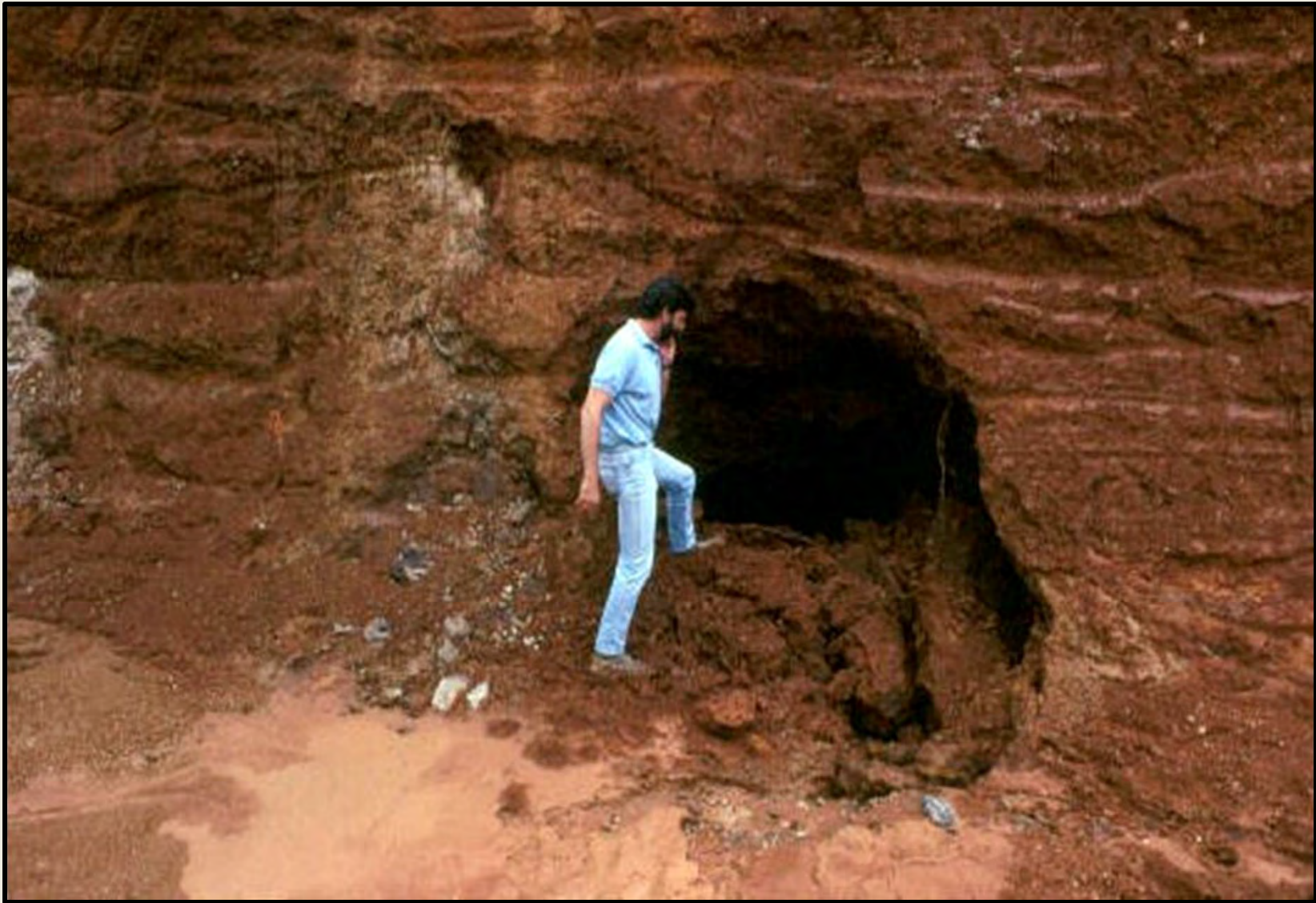
Void in Residual Soil in Karst
