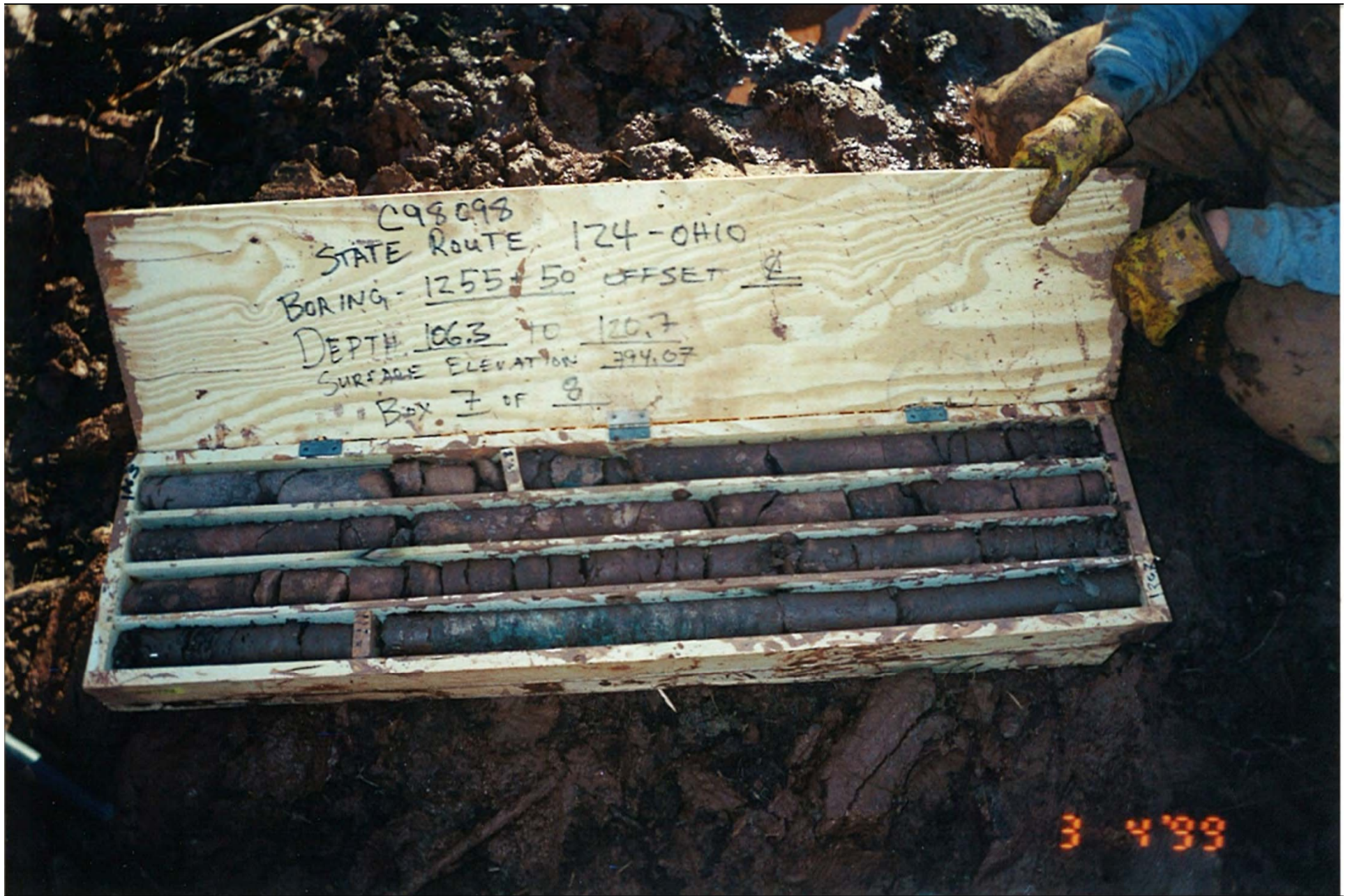
Core Box Containing Redbed Shale Sample
