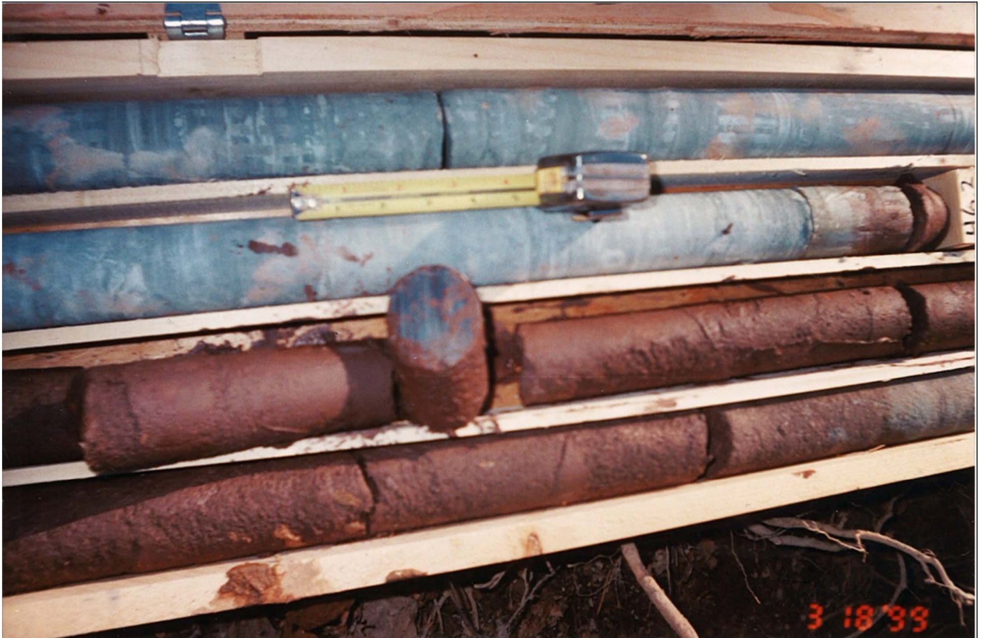
Example of Slickensided Bedrock Surface
