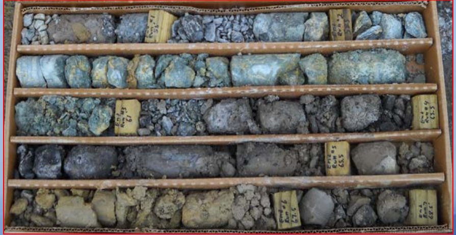
Highly macerated ductile phyllite - breccia from lower Elbrook Typical of basal detachment in Pulaski system exposed in new I81 Climbing lane cuts!
