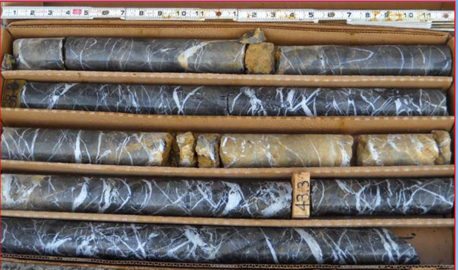
Calcite-filled extension fractures (gash veins) in upper Elbrook dolomite footwall of the Yellow Sulphur fault
