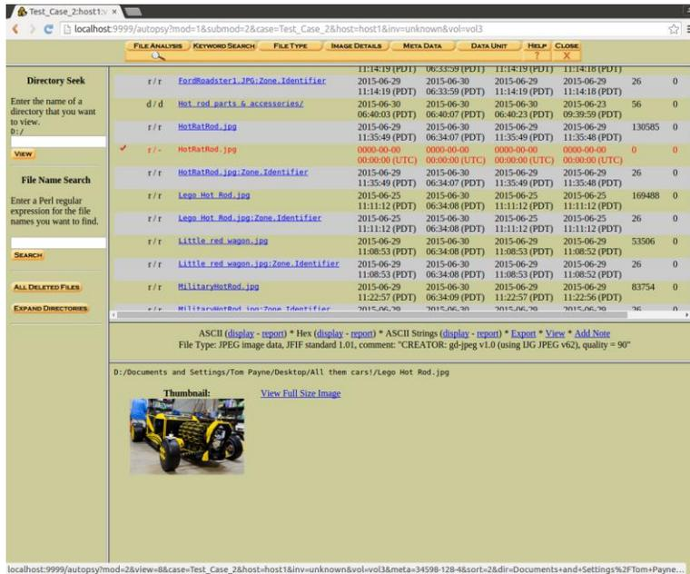
Figure 4: Autopsy™ handling a jpeg image and displaying it
