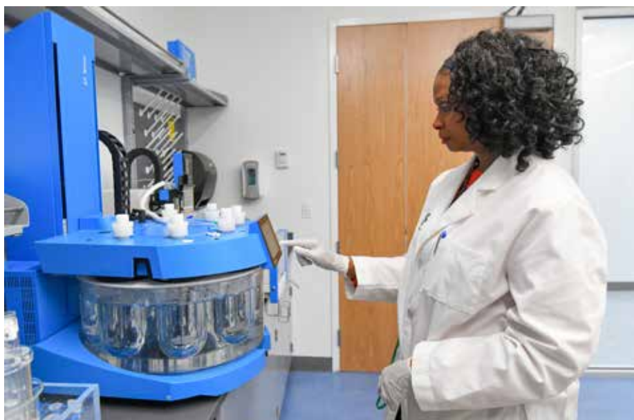
Assistant professor Cynthia Jones, Ph.D. is testing the dissolution profile for a novel solid dosage form on the Sotax AT XTend Dissolution Tester.
