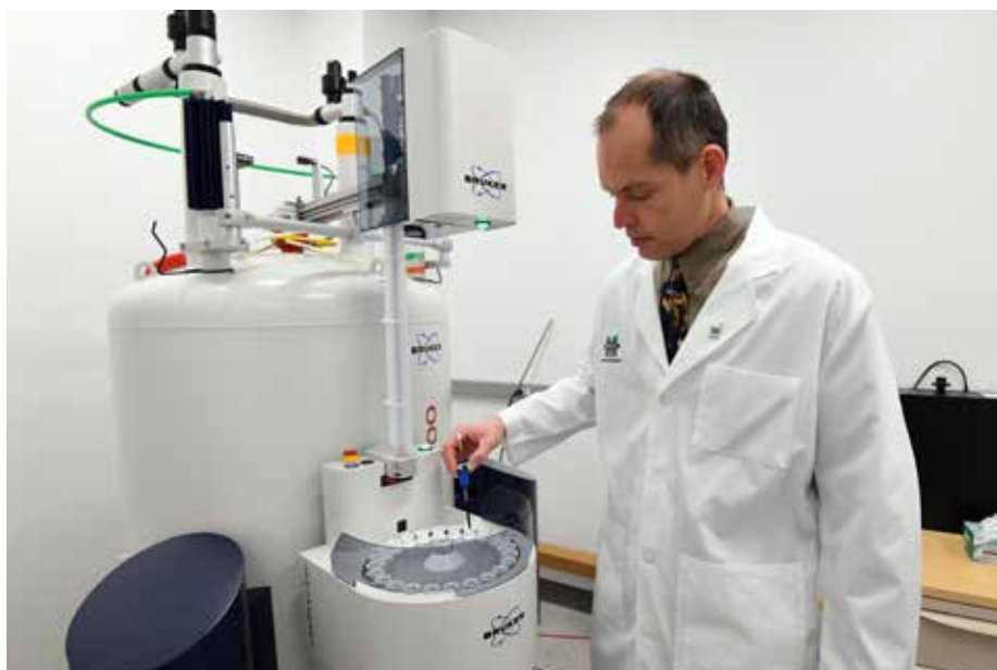
Professor Boyd Rorabaugh, Ph.D., prepares a sample for structural analysis using nuclear magnetic resonance spectroscopy.
